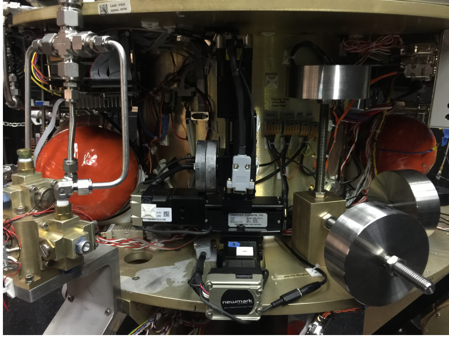
Figure 13: Balancing system installed on the upper stage
